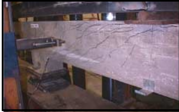
Figure 3. Final failure of beam CW1
