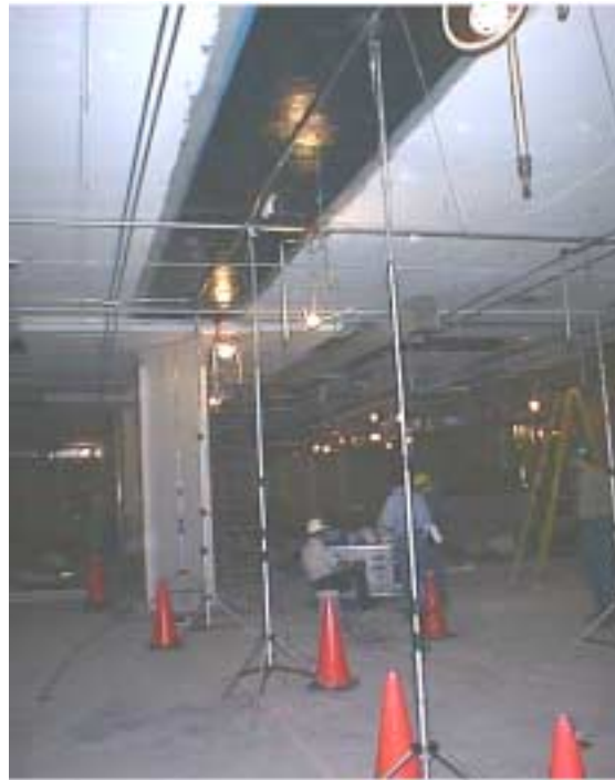
Figure 5: Photograph of instruments to measure deflections used by UMR
